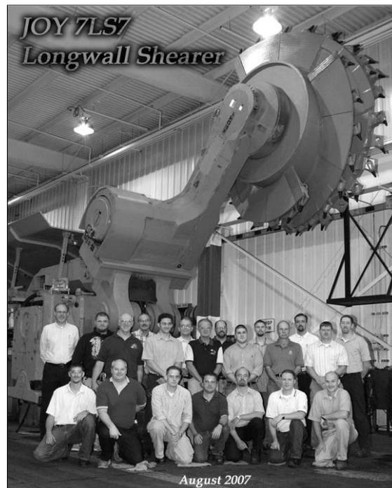
Fig. 1. World's highest shearer 7LS7 at 6.5 metres – China
