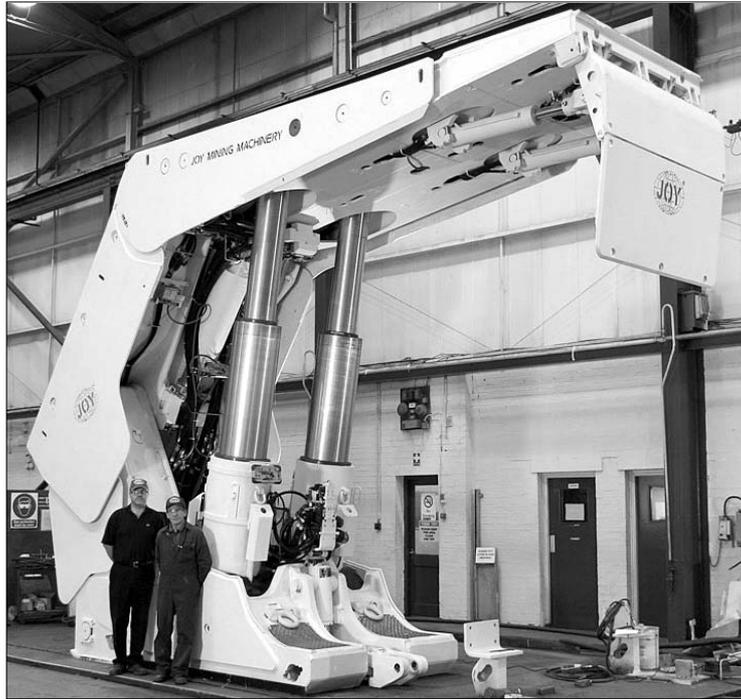
Fig. 2. World's Biggest and Highest Rated Roof Support – 62 tonnes, 90,000 cycles
