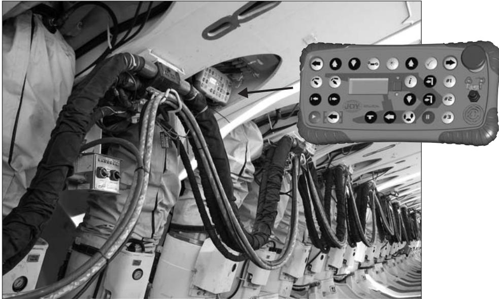
Fig. 3. Full automation of Longwall roof supports with the RS20s Control system
