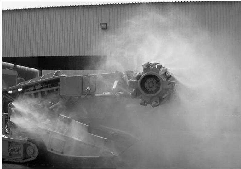
Fig. 7. New 'Wet Head' technology for continuous miners – Water sprays to each cutter pick
