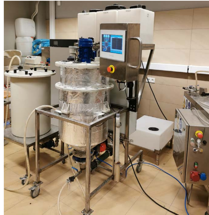
Panek R., Madej J., Bandura L., Słowik G., Recycling of Waste Solution after Hydrothermal Conversion of Fly Ash on a Semi-Technical Scale for Zeolite Synthesis, Materials , 14(6) (2021) 1413
