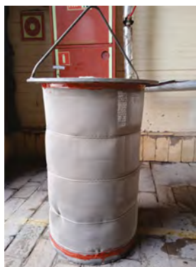
Fig. 4. Filter for the SNK column made of woven sieve
